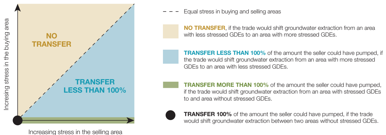
FIGURE 4. Trading ratios could be designed to protect groundwater dependent ecosystems. 320 For example, proposed transfers of groundwater extraction allocations to buyers in areas with more stressed groundwater dependent ecosystems (GDEs) could be barred to avoid increasing the stress on those GDEs. On the other hand, a transfer from an area with stressed GDEs to an area without stressed GDEs might entitle the buyer to pump more groundwater than the seller could have pumped, while a transfer to an area with less stressed GDEs might be allowed to go forward, but might entitle the buyer to pump less than the seller could have pumped.
